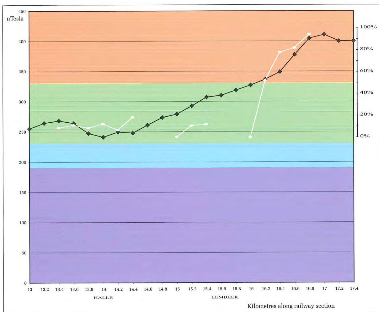
Figure 30: Profile along the railway section of the average aeromagnetic field values (black line), expressed in nTesla relative to the regional average. Note the increase towards the south. The magnetic susceptibility of the rocks determined qualitatively at outcrop level, as discussed in Figure 8, are indicated as a white line. The latter series is scaled (scale bar on the far right) to make the minima and maxima of both series correspond, in order to emphasize the relation between outcrop and remote sensing data. Background colours as on the aeromagnetic map in Figure 32.
