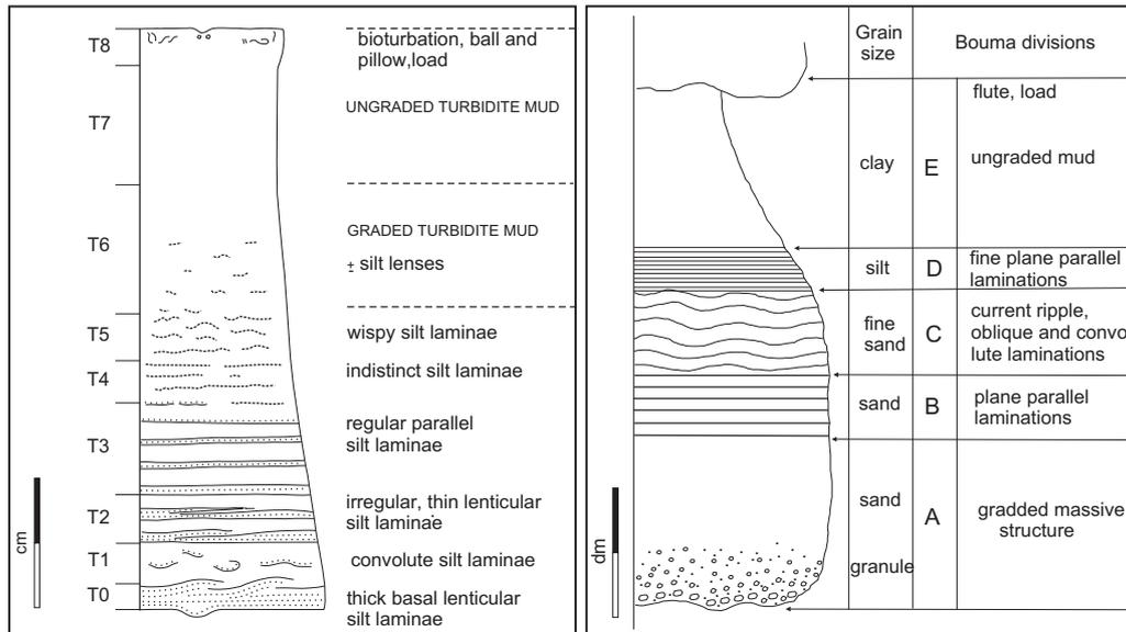
**Figure 20.** High-density turbidite model (Bouma model, at right) compared with low-density turbidite model (Stow model, at left): note the difference in scale between the two models.
