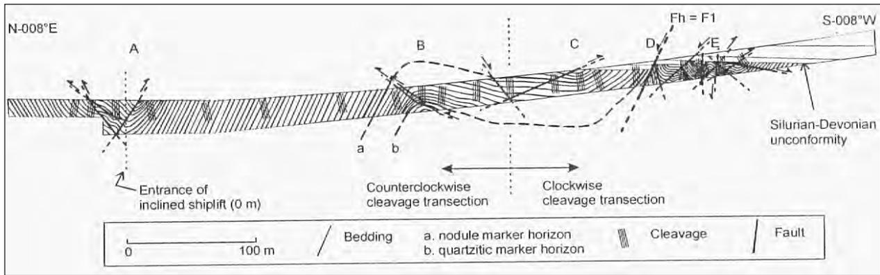
**Figure 36.** Section along the E-side of the inclined shiplift of Ronquières. A, B, C, D and E are respectively the Porte Avale synform, the central antiform, the Belvédère synform, the faulted antiform and the synform complex. The unconformity is at the southern extremity of the section. From Debacker et al. (1999).
