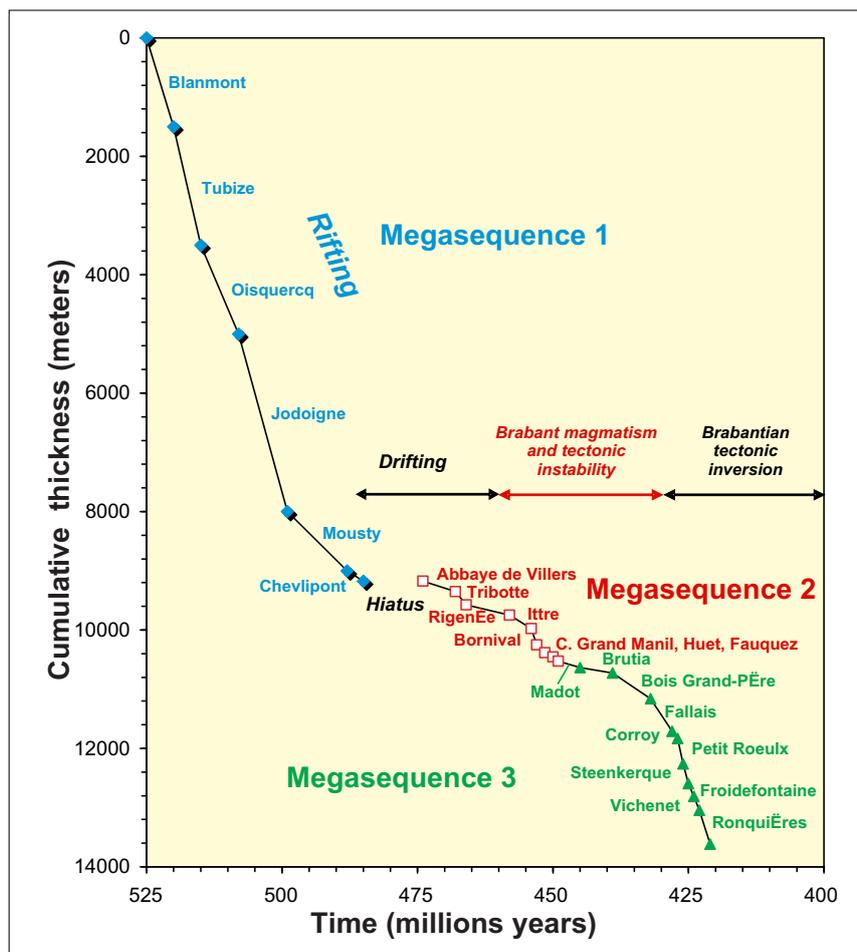
**Figure 7.** Cumulative thickness curve of the Lower Palaeozoic sediments of the BM plotted against the stratigraphic age (thickness from Herbosch & Verniers, 2013, 2014 and for the Silurian from Verniers et al., 2001).
