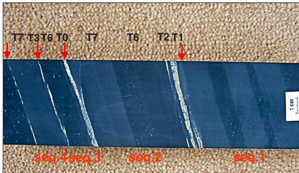
**Figure 35.** Polished surface of a core showing sequences of mud turbidite (red arrows) and the divisions of the Stow model (in black). Lessines borehole 149 m (Herbosch et al., 2008). Pyrite (in yellow) underlines the base of each sequence. Compare with the model of Fig. 20.
