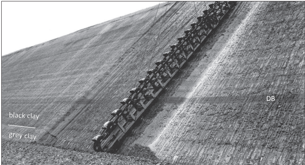
Figuur 36. Photograph of the Boom Clay in the Putte clay pit. The height of the excavation wall is 16.5 m. The prominent dark grey layer about 6 m above the base of the pit is the double layer (DB) consisting of only one layer with very high silt/clay fraction ratio having only a faint separation in the middle. The indicated boundary between grey and the black clay near the base of the pit is the limit between the Terhagen-Putte Members.
