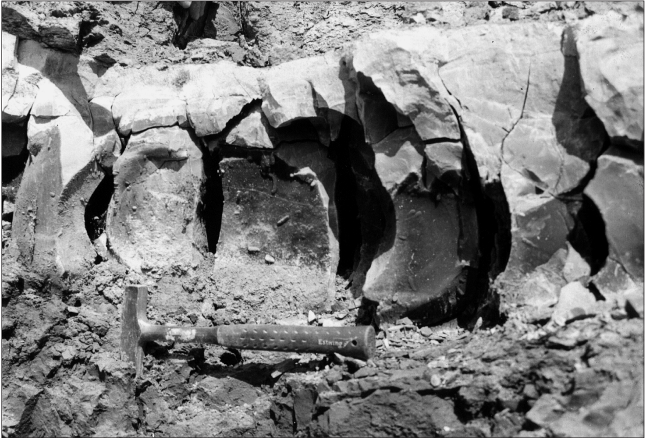
Figuur 48. Septarian fractures in a carbonate concretion from the S20 level within the Boom Clay. The vertical cracks are wide open in the center and thin and bulge out towards the outer boundary of the concretion where they disappear. Quarry at Terhagen (from De Craen, 1998).
