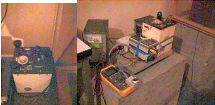
Figure 12. Pictures of the LaCoste without a triangular base (at left) and with a triangular base (at right), taken at the fundamental reference point of the Belgian network.
