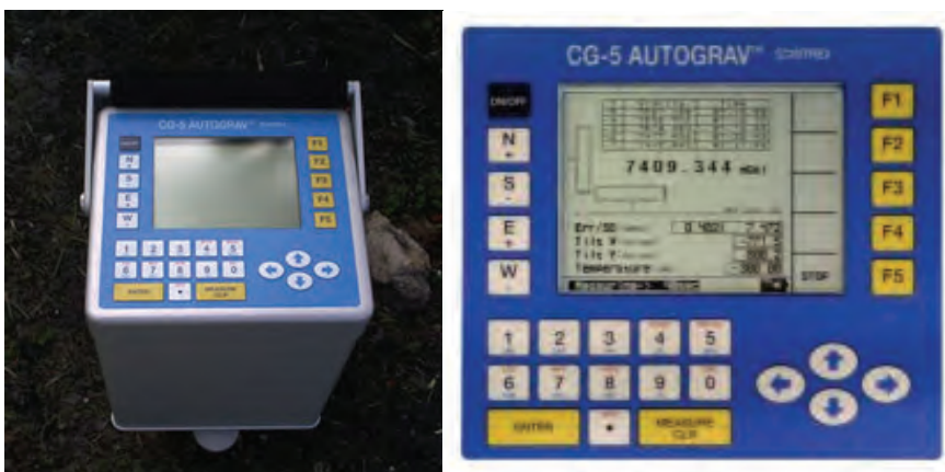
Figure 17. The Scintrex CG5 gravimeter, with a zoom-in on the interface; the reading is in mGal.
