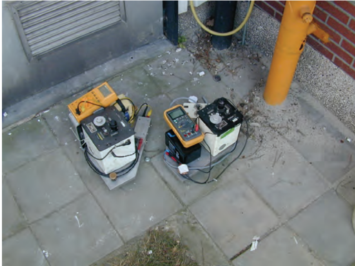
Figure 14. Instrument setup for measurement in the field. Notice the spotting nail between the instruments.
