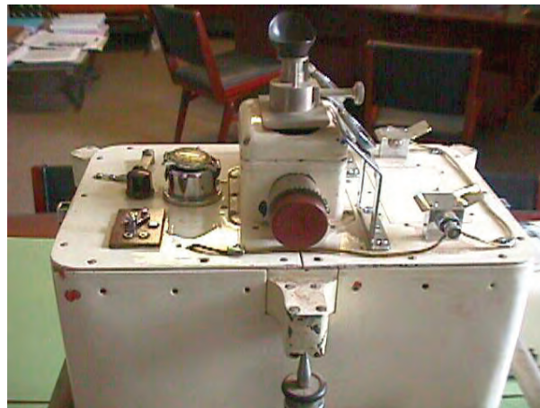
Figure 20. Two views of the Norgaard 256 gravimeter, acquired in 1946.
