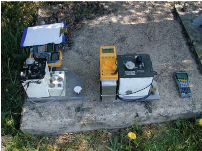
Figure 13. Gravimeters set up for field work. At left the G402 (ROB) and at right the D 32 (MGI), both fixed on a triangular base. To the right of the instrument there is a digital recorder. Above left a field notebook to help the operator to check the behaviour of the meter.
