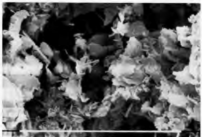
Fig. 3. – SEM-photograph of subsample 88A27 after a 24 hours compaction test at 0.5 \text{ kg/cm}^2 (White bar on photograph is 10 \mu\text{m} ; pore space is indicated by arrow).
