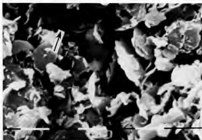
Fig. 4. – SEM-photograph of subsample 88A27 after a 24 hours compaction test at 4 kg/cm 2 (White bar on photograph is 1 µm; pore space is indicated by arrow).
