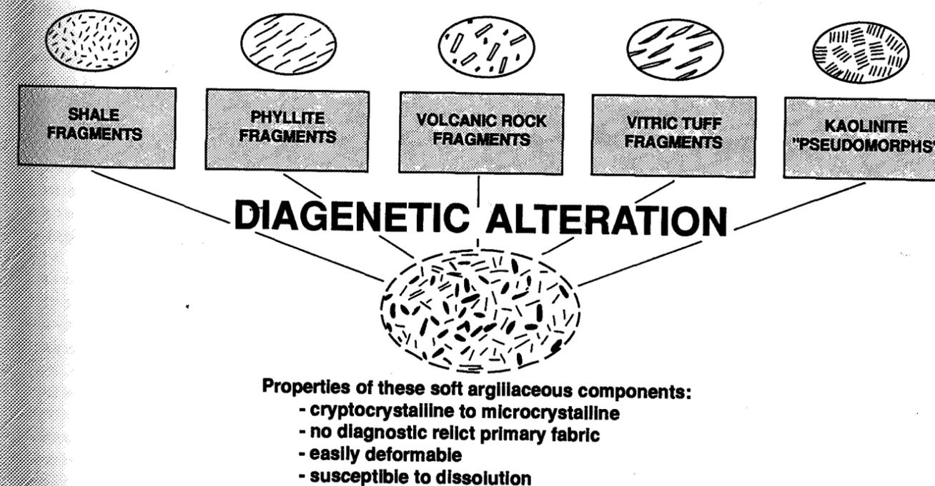
Figure 3. Mineralogically unstable clasts in clays, shales and sandstones, an often-neglected, but important component of sedimentary rocks.
