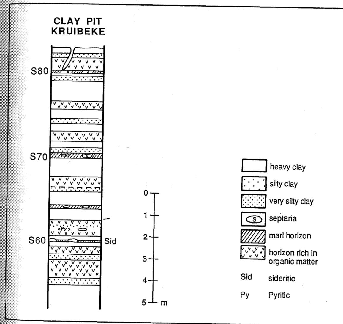
Figure 2. Composite Boom Clay section, northern Belgium (after Vandenberghe & Van Echelpoel, 1987).
