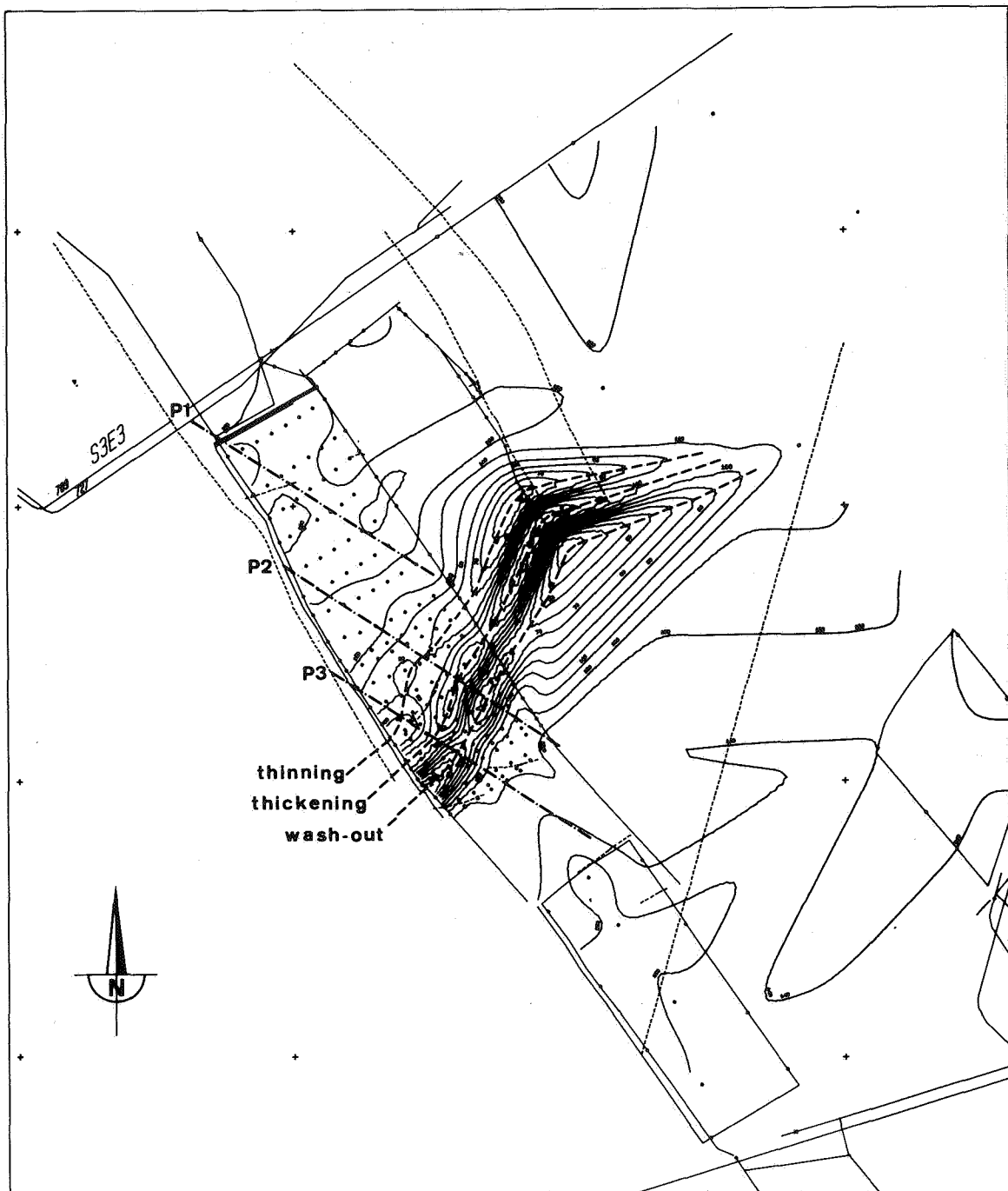
Figure 29. Computer-generated isopach map of coal seam 66-67-68 affected by a wash-out, in a new panel located about 1 km to the east of the former studied area (figures 27, 28). Lines P1 to P3 correspond to cross-sections of figure 30.
