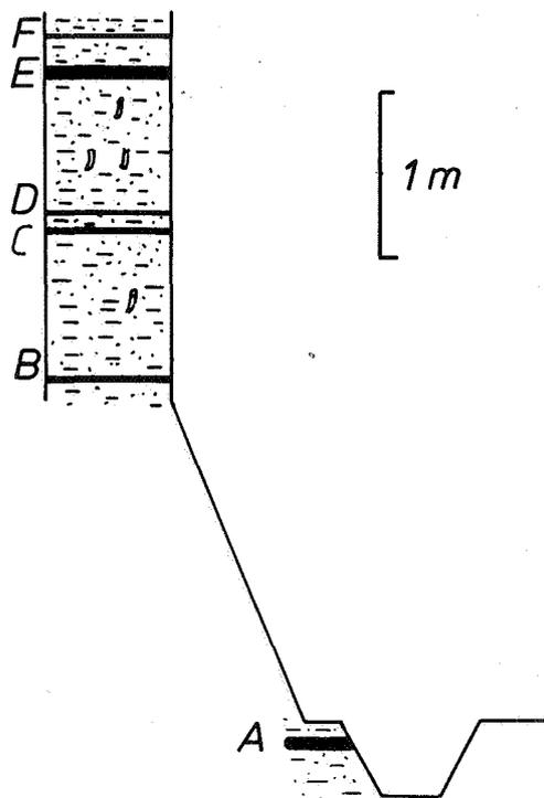
**Figure 3:** Section of the railroad trench at Schoonboeke. The Mont Panisel Member is exposed, with 5 sandstone layers (A - F).
