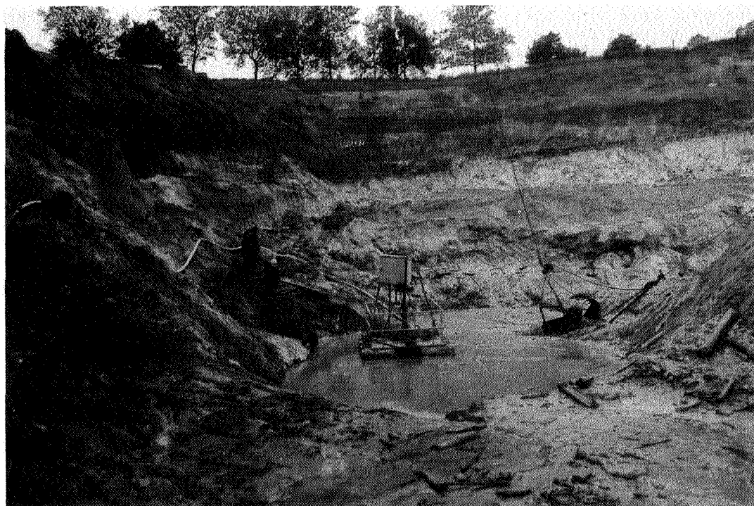
Fig. 3. View of Fleurus open-pit exploitation (June, 1980). Contact between the baritic body (light grey) and the overlying Caenozoic formations (dark grey).
