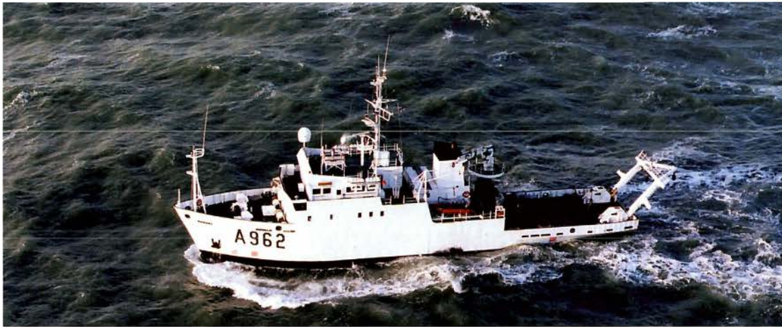
The Belgica is 50.9 m long and 10 m wide. Its cruising speed is 12 knots (22 km/h), which allows it to travel 5000 miles in 20 days.
