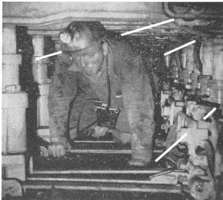
PILES HYDRAULIQUES DE SOUTÈNEMENT MARCHANT
