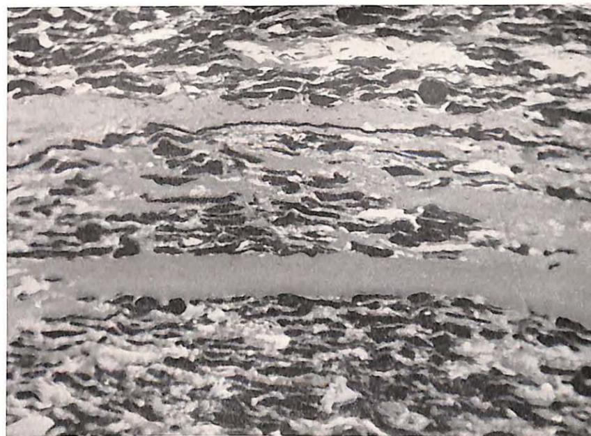
Figure 7. — Mélange vitrain-durain (crassidurain), charbon flambant.
