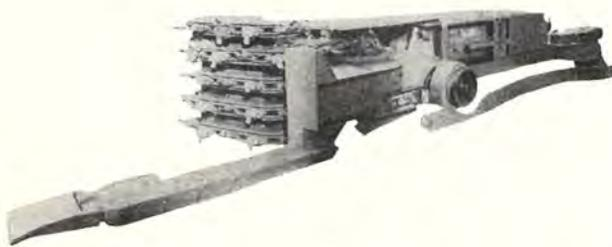
Fig. 71. — Dauerwühler ou Continuous Miner Eickhoff.
