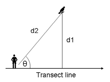
Fig. 4. d1 (perpendicular distance) can be calculated using d2 and the sighting angle  $\theta$  (d1=d2\*sin( $\theta$ )).
