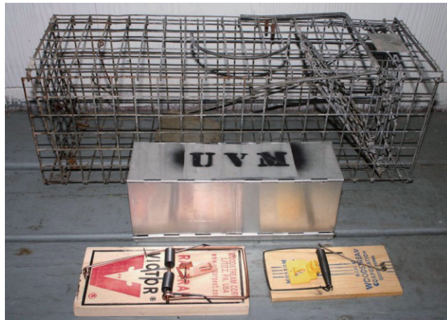
Fig. 1. Popular trap types. Back: Collapsible Tomahawk trap for squirrels, small carnivores, and large rats. Centre: Standard-sized collapsible Sherman trap. Front left: Victor Rat trap. Front right: Museum Special snap trap. (Photo by Jan Decher).
