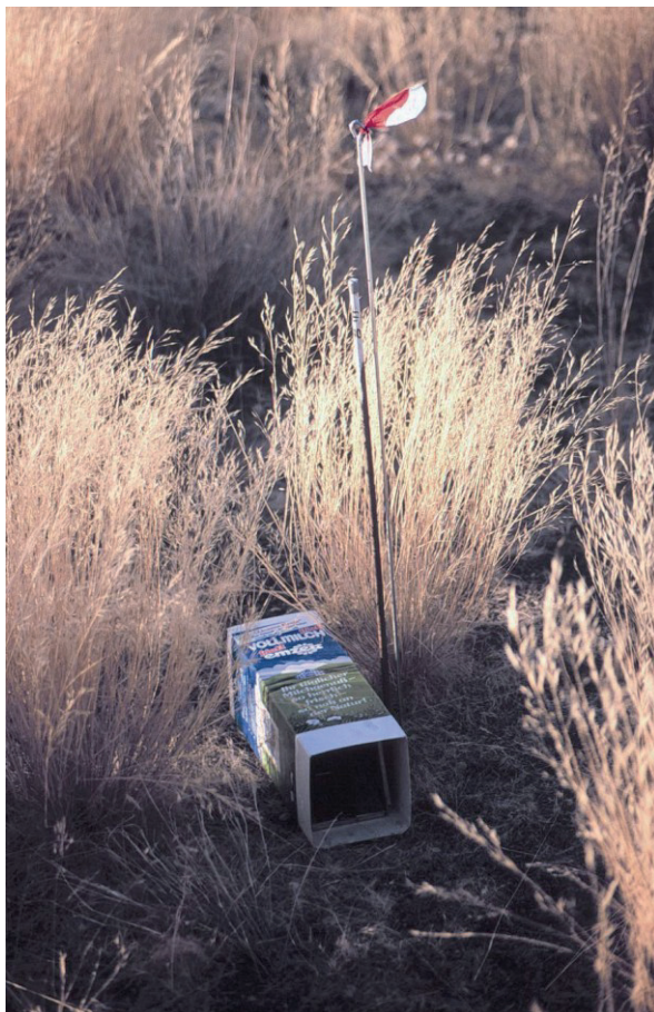
Fig. 2. Standard Sherman Live Trap (LFA-TDG, 7.5 x 9 x 23 cm) protected in a 2 litre milk carton. (Photo by Anke Hoffmann).
