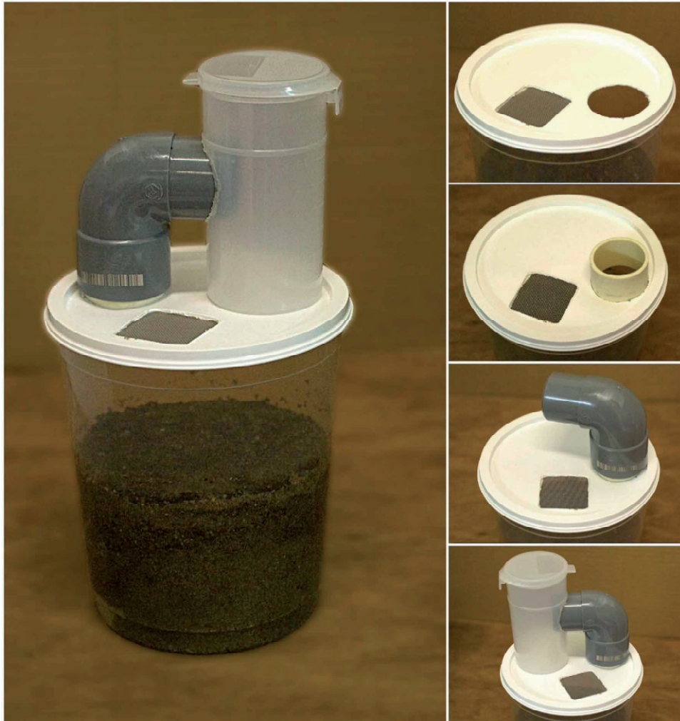
Fig. 8. Collecting jar of an emergence trap made of plumbing tubes. No glue is needed to fix the separate parts except for the mesh. (Photos by Filip De Block).
