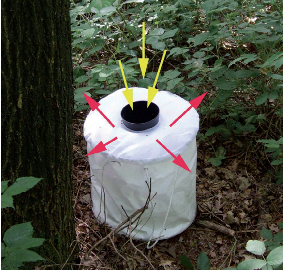
Fig. 10. The BG-Sentinel suction trap was originally designed to collect mosquitoes. The arrows indicate the convection stream with yellow arrows corresponding with the air that is sucked in, and red arrows showing the air stream carrying the odours of the lure out of the trap. Due to its white colour many pollinators are collected. (Photo by Wouter Dekoninck).
