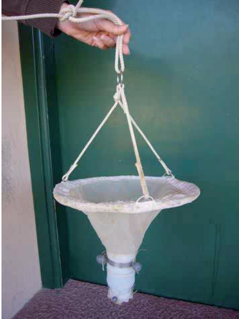
Fig. 9. A modified version of the Cvetkov net, adapted to sample in shallow wells. (Photo by Damia Jaume).
