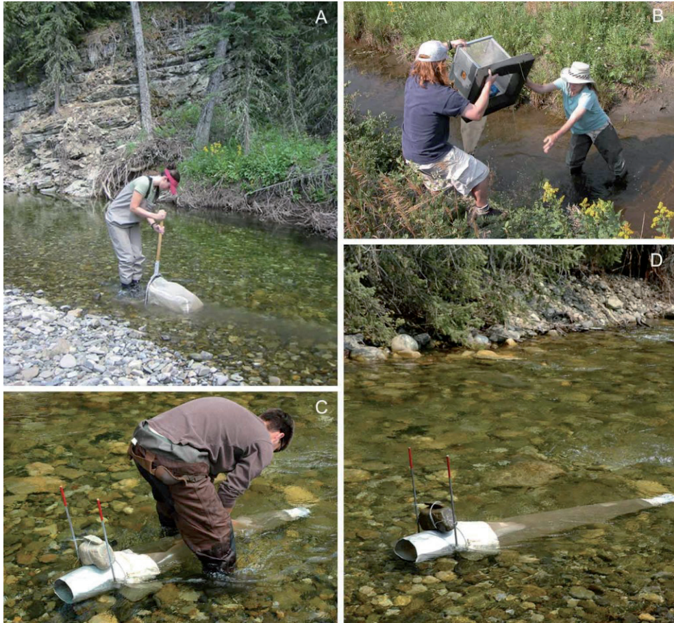
Fig. 6. Sampling macroinvertebrates. A. Kick-sampling with D-net in Alberta, Canada; B. Sampling a stream in Saskatchewan, Canada; C. Setting up drift net in stream in Alberta, Canada; D. Drift net in stream Alberta, Canada. (Photos by Heather Proctor)
