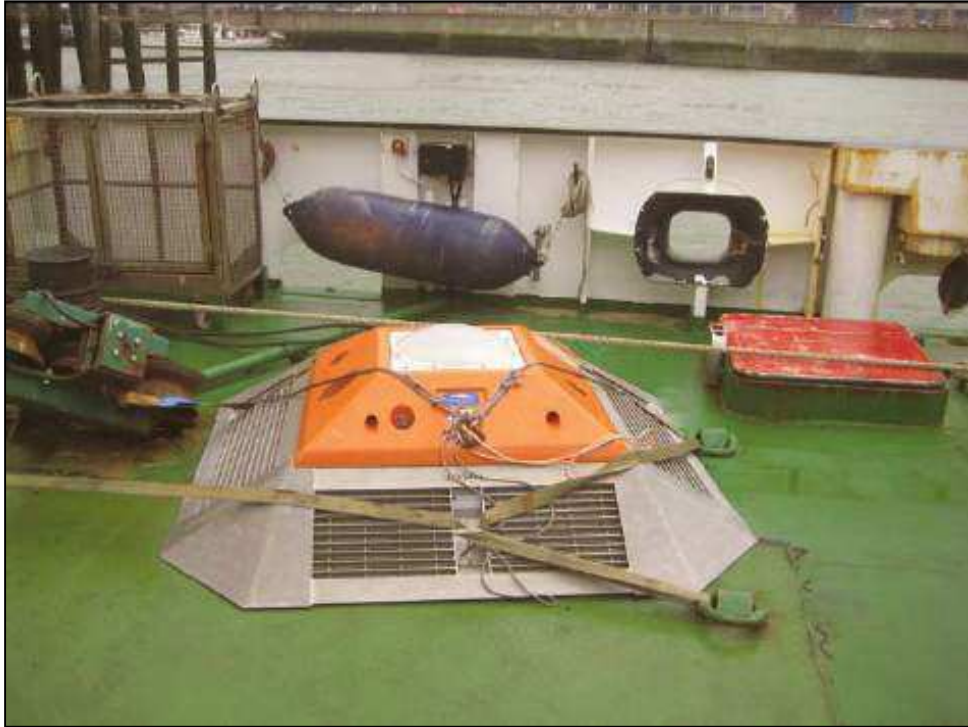
Figure 3: Bottom mounted ADCP.
