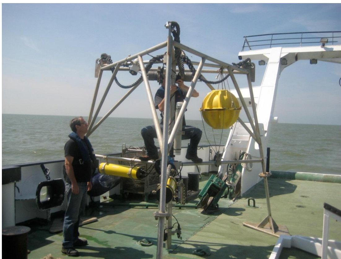
Figure 6.1. Tripod as used to deploy the underwater noise recorder to the seabed
