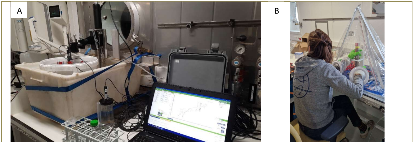
Figure 1: (A) sediment oxygen profiles measured on board RV Belgica with microsensors and (B) extraction of porewater and slicing of sediment cores in an oxygen-free glove bag
