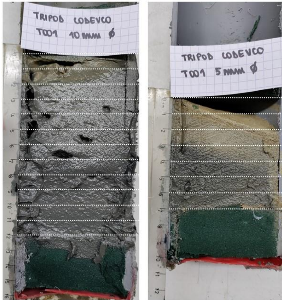
Figure 2.22. Pictures of the two sediment traps collected on tripod T001. The dotted white lines indicate the one-centimeter slices analyzed in the Malvern.
