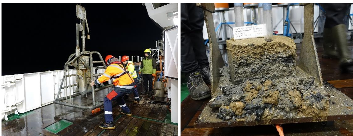
Figure 2.9. Pictures of the box core (left image) and of the subsampling (right image).
