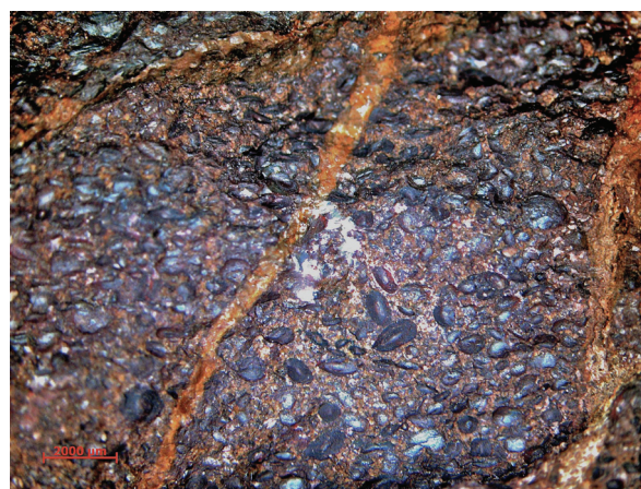
Fig. 5 – Lower Famennian OIS, Hodimont Formation, Lambermont (Belgium). Large hematitic ooids and flattened micro-oncoids in a red-stained carbonate matrix. Macroscopical view of rough surface. Scale bar is 2 mm.
