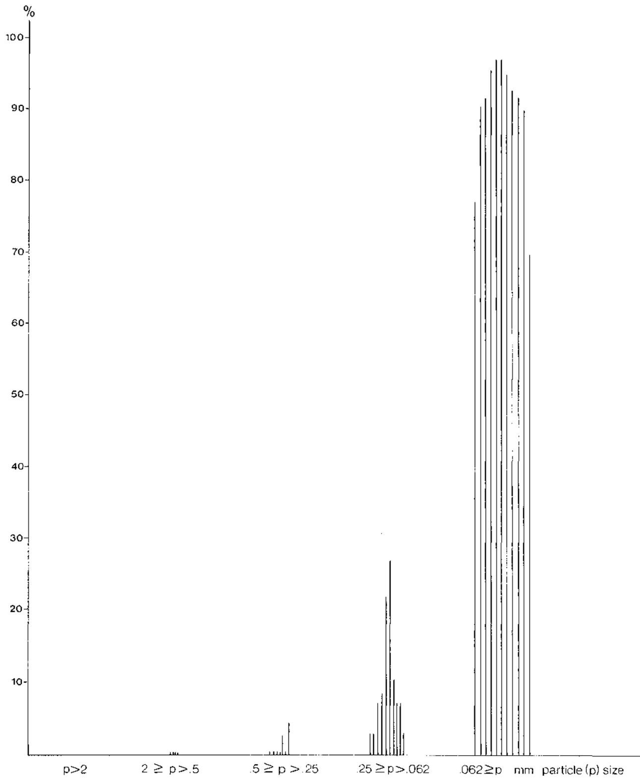
FIG. 60. — Grain size distribution of clays.
