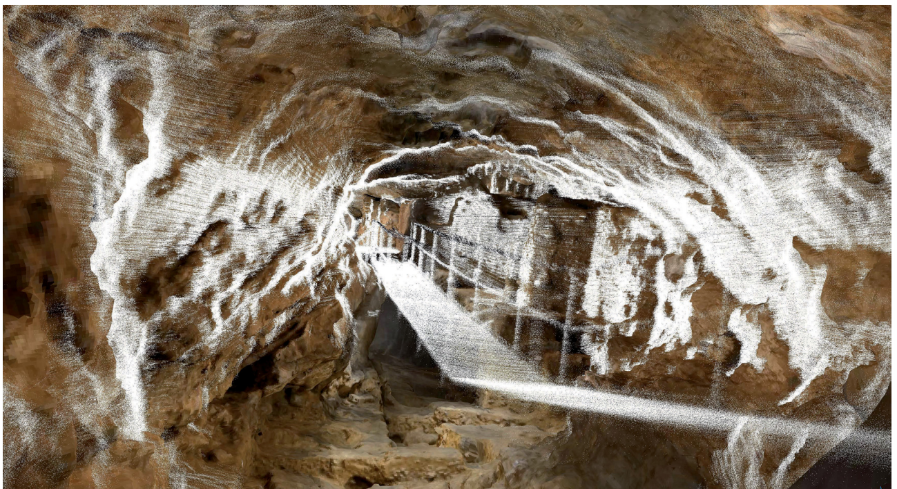
Fig. 4 – Superposition of LiDAR and UAV 3D data within the Scladina Cave.
