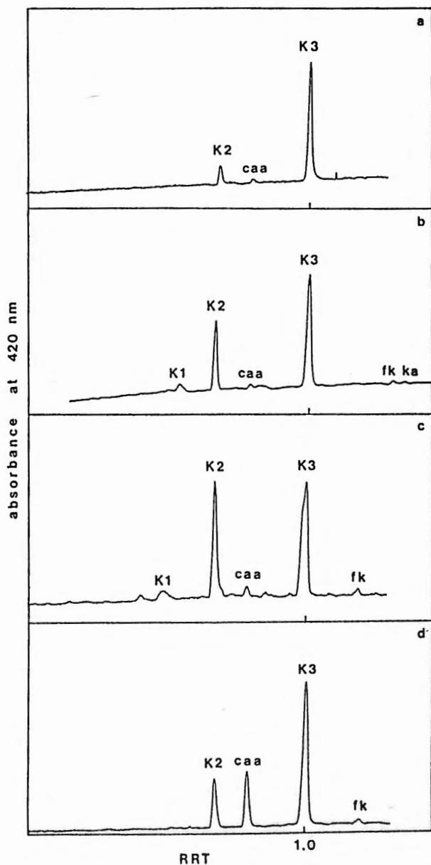
Fig. 4. — HPLC of Kermesidae pigments, recovered from dyed wool, monitored at 420 nm. (a) : *Kermes ilicis*; (b) : *Kermes biblicus*; (c) : *K. palestiniensis*, unstriped specimen; (d) : *K. palestiniensis*, striped specimen. The abbreviations refer to table 2. RRT : retention time, relative to K3 (RRT of K3 = 1.00). Small variations in RRT of fk and ka in (b) are due to modification of the elution program.
