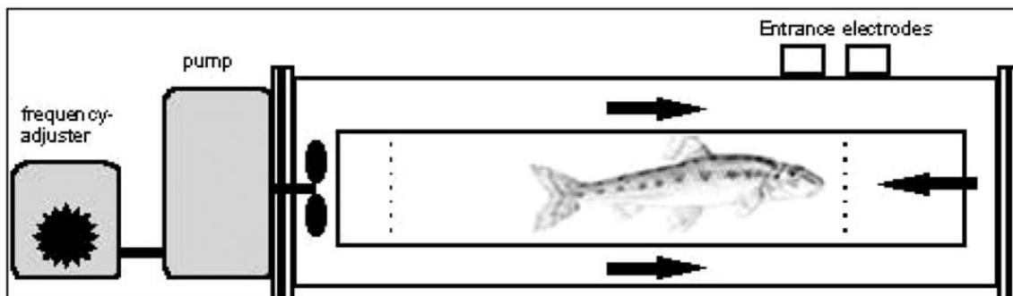
Fig. 2. – Schematic figure of the respirometer. The black arrows indicate water flow, the dotted lines represent membranes, which keep the fish in the inner tube and allow water to flow through the inner tube.
