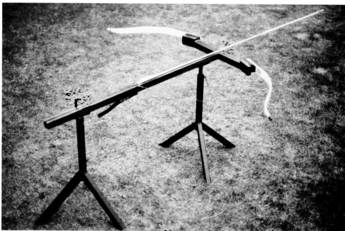
Fig. 1 — The firing apparatus used in the experiments spanned and ready for use (Photographs by the author).
