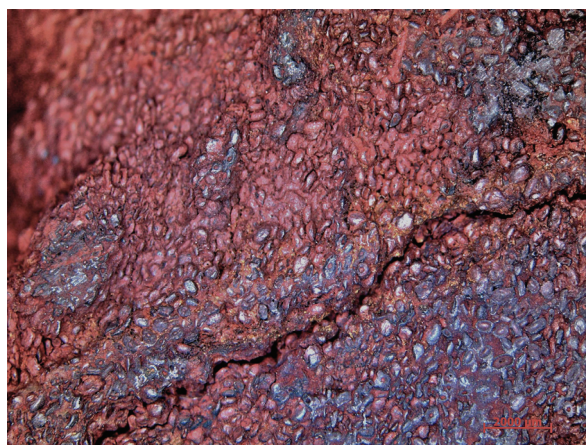
Fig. 4 – Ordovician OIS, Urville Shales Formation, Urville (Normandy, France). “Flax seed” ore facies. Weathered hematitic ooids. Macroscopical view of weathered surface. Scale bar is 2 mm.
