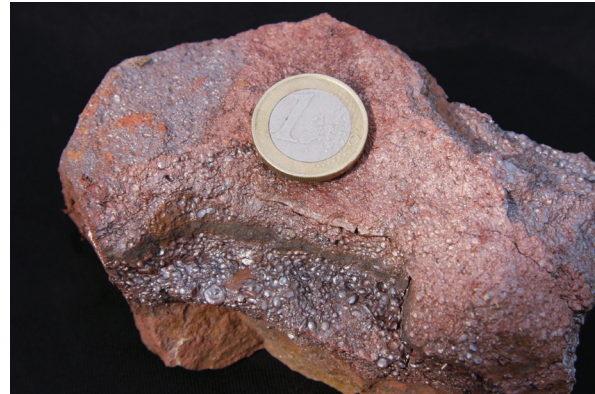
Fig. 6 – Lower Famennian OIS, Hodimont Formation, Huy (Belgium). Mixed, "flax seed" ore and fossil ore facies. Medium-sorted hematitic coated grains and rounded bioclasts on a bedding surface. Macroscopical view of rough surface.
