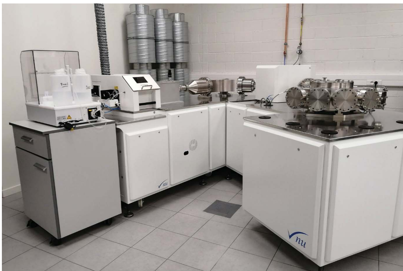
Fig. 2 – The new Nu Instrument PLASMA 3 MC-ICP-MS of the BB-LAB funded by the European Union’s Horizon 2020 Research and Innovation programme under grant agreement 948913 (ERC Starting Grant LUMIERE). This MC-ICP-MS is fully dedicated to the study of plant, animal and human remains.
