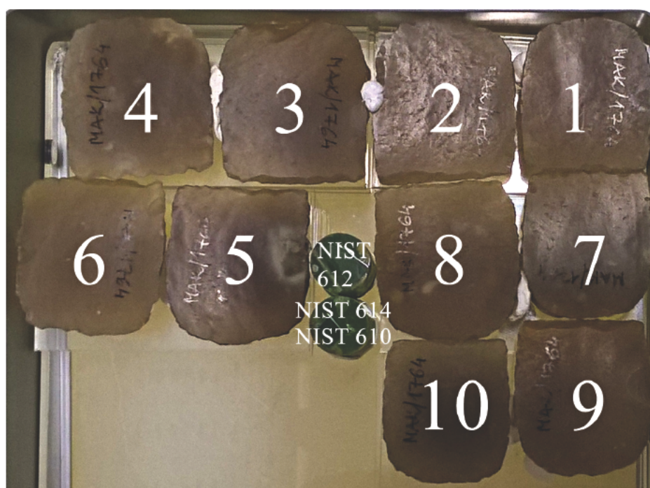
Fig. 4 – Mount for LA-ICP-MS analysis containing the sample of investigated gunflints. Photo: M. Brandl.
