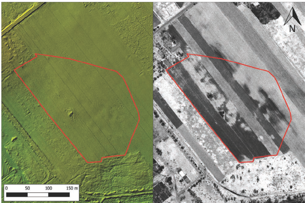
Fig. 1 – Chocolate flint mining field 'Przyjaźń' in Rzeczków, Radom district. Comparison of digital terrain model (a) and visualisation showing intensity of laser return beam (b) on the site with a ploughed surface. The line is indicating the area where flint artefacts are present.
