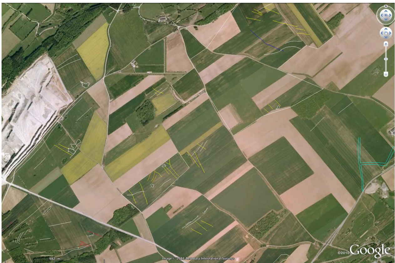
Figure 7 : Familles de diaclases/failles et linéaments lithologiques sur le Gerny (recensement non exhaustif). – Sets of joints/faults and lithologic lineations on the Gerny plateau (non-exhaustive survey).
