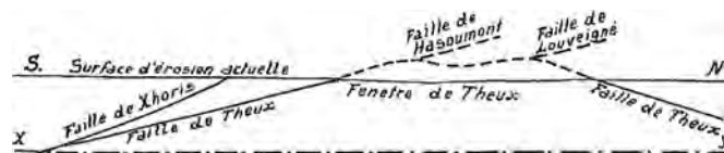
Fig. 113. S-N cross-section sketch showing the relationship between the Xhoris and the Theux faults (Fourmarier, 1928b).
