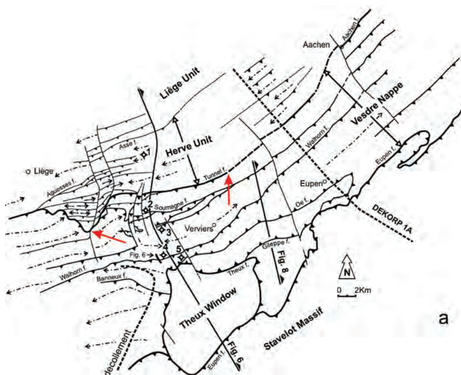
Fig. 89. Structural units and faults in northeastern Belgium and Germany (Hance et al. , 1999). Main fold axis, plunge directions and main deep boreholes are also given. 1-2. Pépinster. 3. Soiron. 4. Soumagne. 5. Bolland. Red arrows show the Tunnel Fault as considered in this paper.
