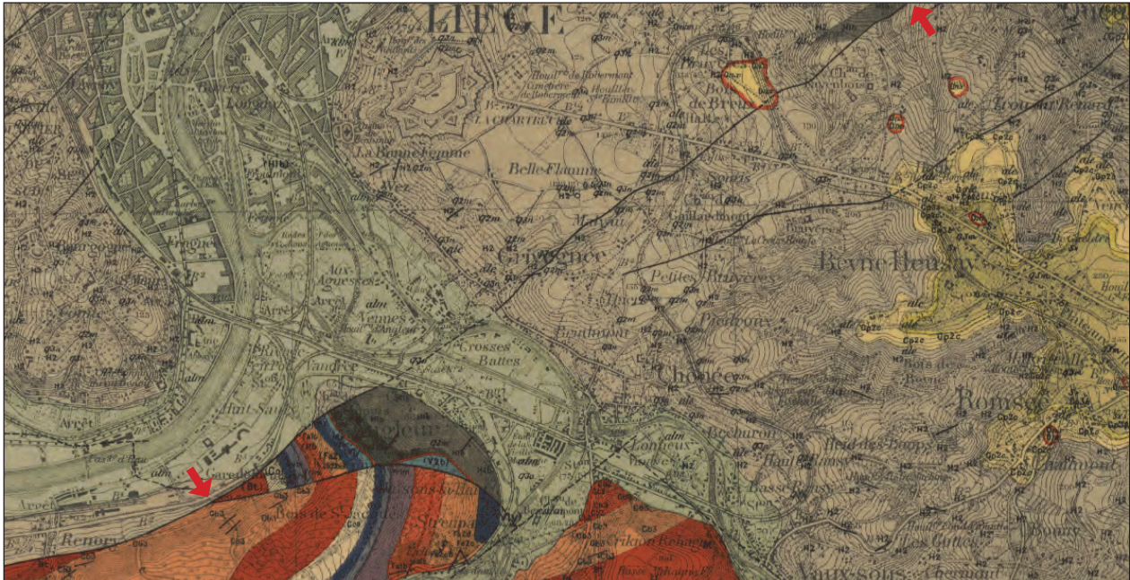
Fig. 10. Extract of the geological map of Seraing – Chênée (n°134; Forir, 1897). Arrows indicate the western segment of the Aguesses-Asse Fault traced over 8.4 km.
