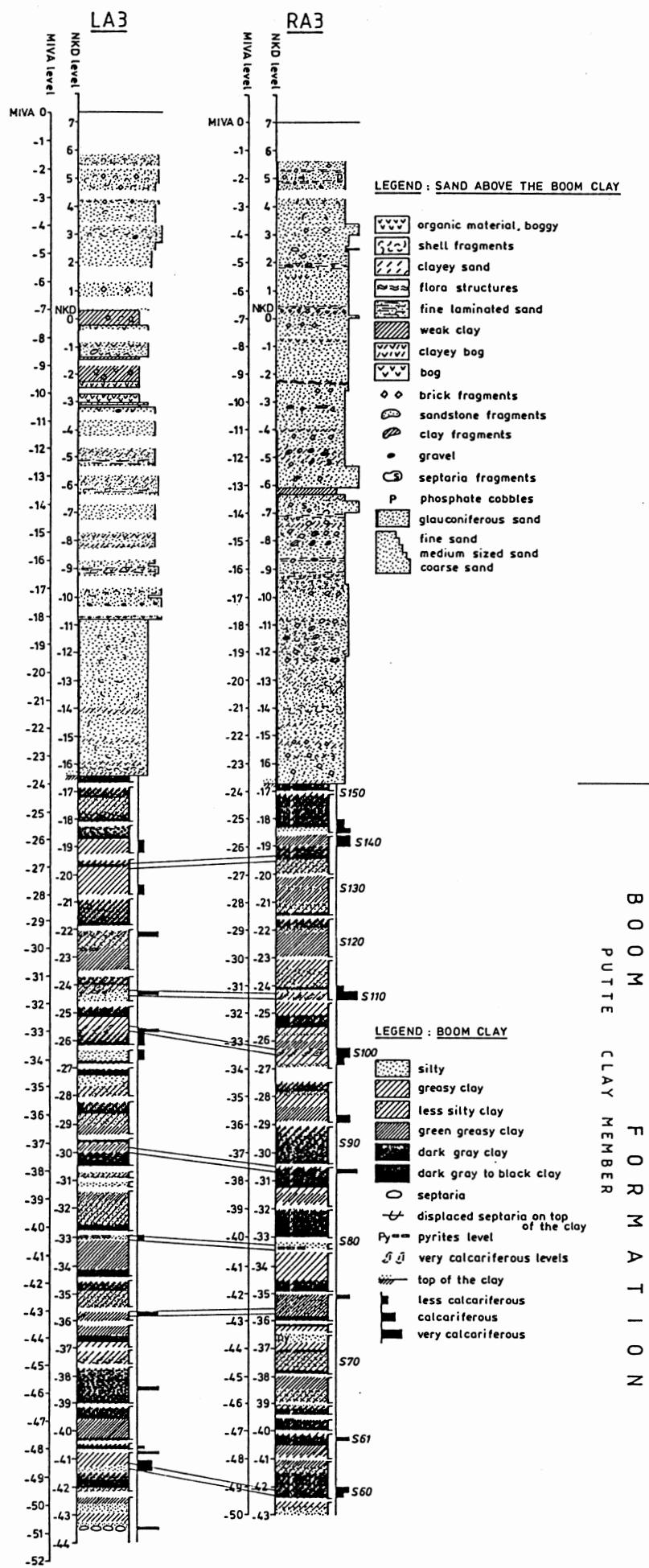
Fig.4 : Logs of the wells LA 3 (= 28W - 627) and RA 3 (= 28W - 626)
