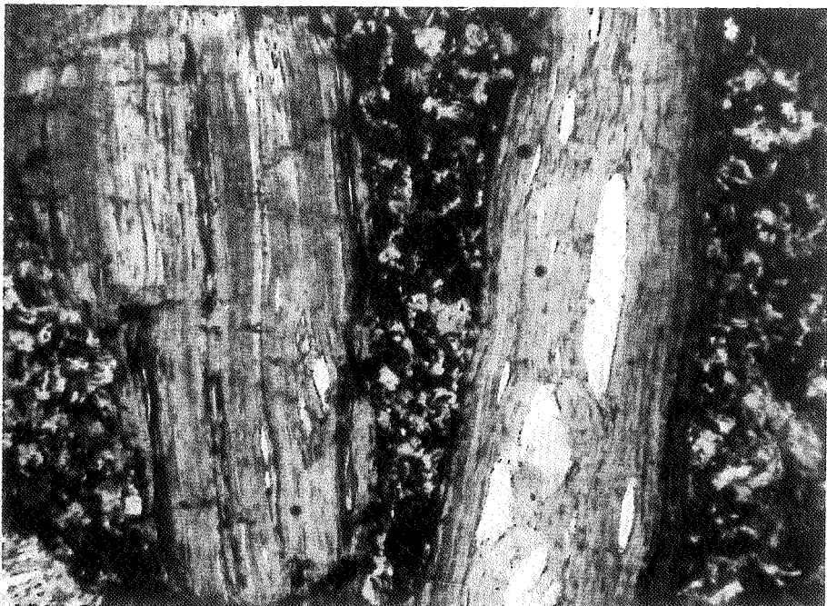
Photo 3 - Nodule 2: chlorite phenocrysts containing lenses of monocystalline quartz between the cleavages. (40 x).
