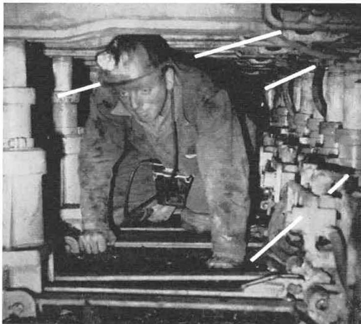
PILES HYDRAULIQUES DE SOUTÈNEMENT MARCHANT
