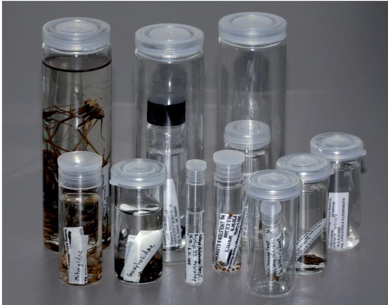
**Fig. 2.** Handling Glass vials are not a good choice for storing specimens during field work as they are heavier and less safe than plastic vials. (Photo by authors).
