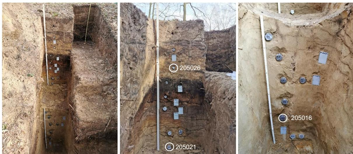
Fig. 2 – Picture (left) of the complete sampling pit and close-ups (center and right) of the two profiles in the sampling pit. The analyzed OSL samples are marked with white circles and their corresponding GLL-code.
